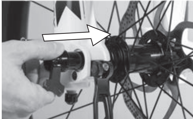
Figure 25: Pushing the axle into the hub
