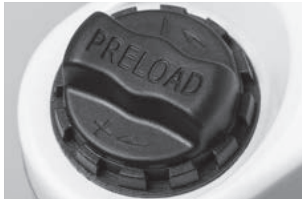
Negative deflection setting wheel on the suspension fork crown
