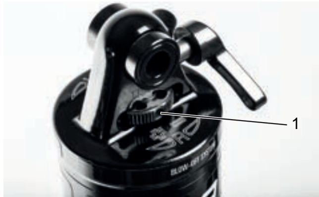
Figure 54: Suntour rebound adjuster wheel (1) on the rear frame damper
